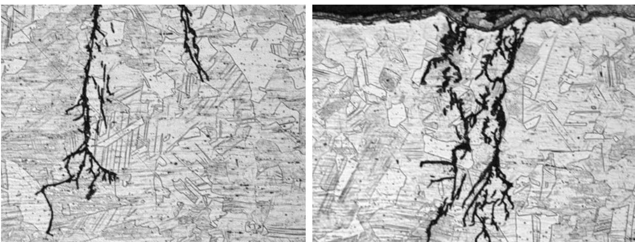
Figure 5: Etched metallographic sections after etching per ASTM A262 and appearance of a step structure.
